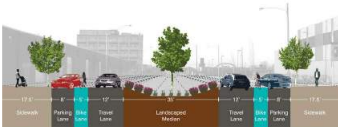
Street section showing proposed American Street green median improvements from Lehigh to Indiana
